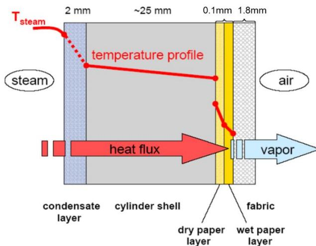
Figure 19: heat flux from steam through the shell of the dryer can to the paper
