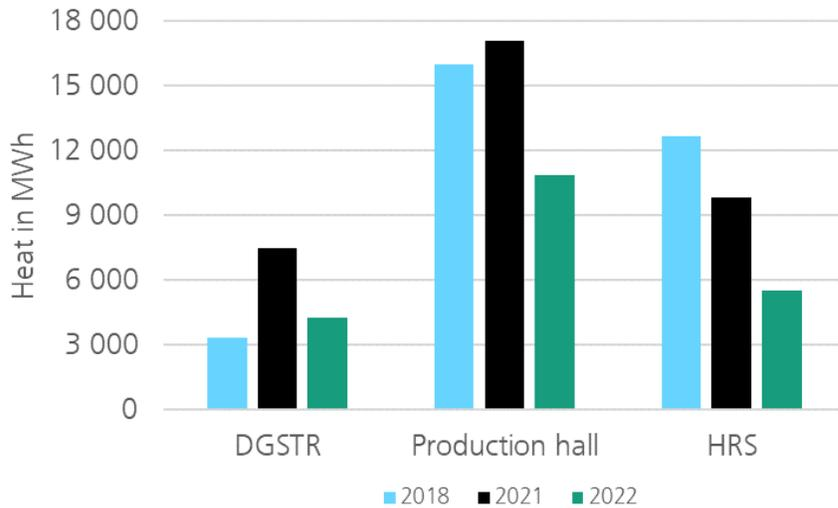
**Figure 13: Annual heat demands for Back-up heat exchanger (DGSTR), heat consumers (Production hall) and Heat Recovery System (HRS)**
