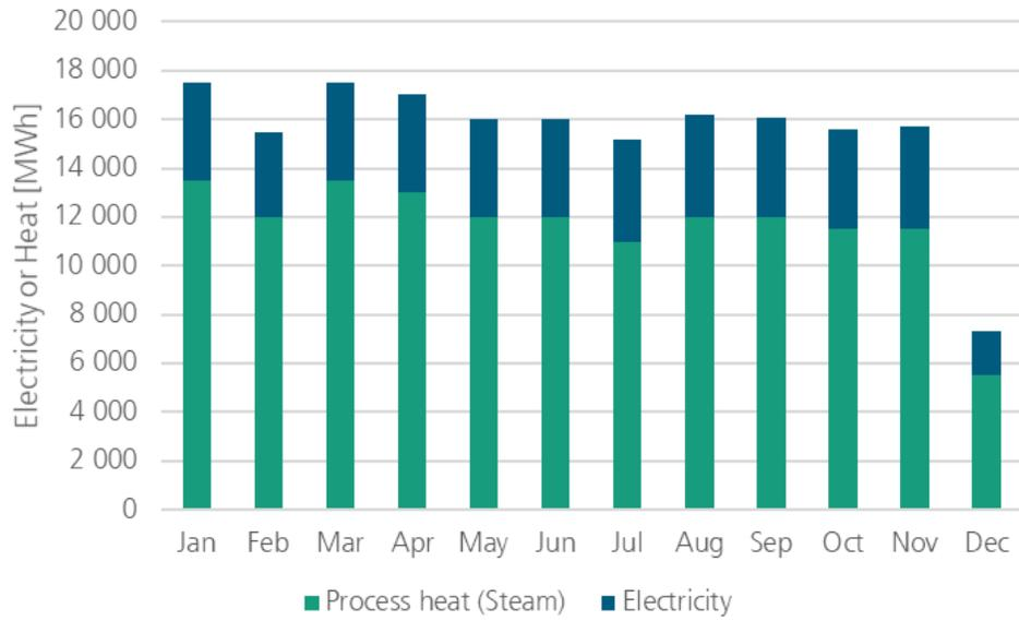
**Figure 7: Monthly energy demand for process heat (steam) and electricity for the paper production in the year 2019**
