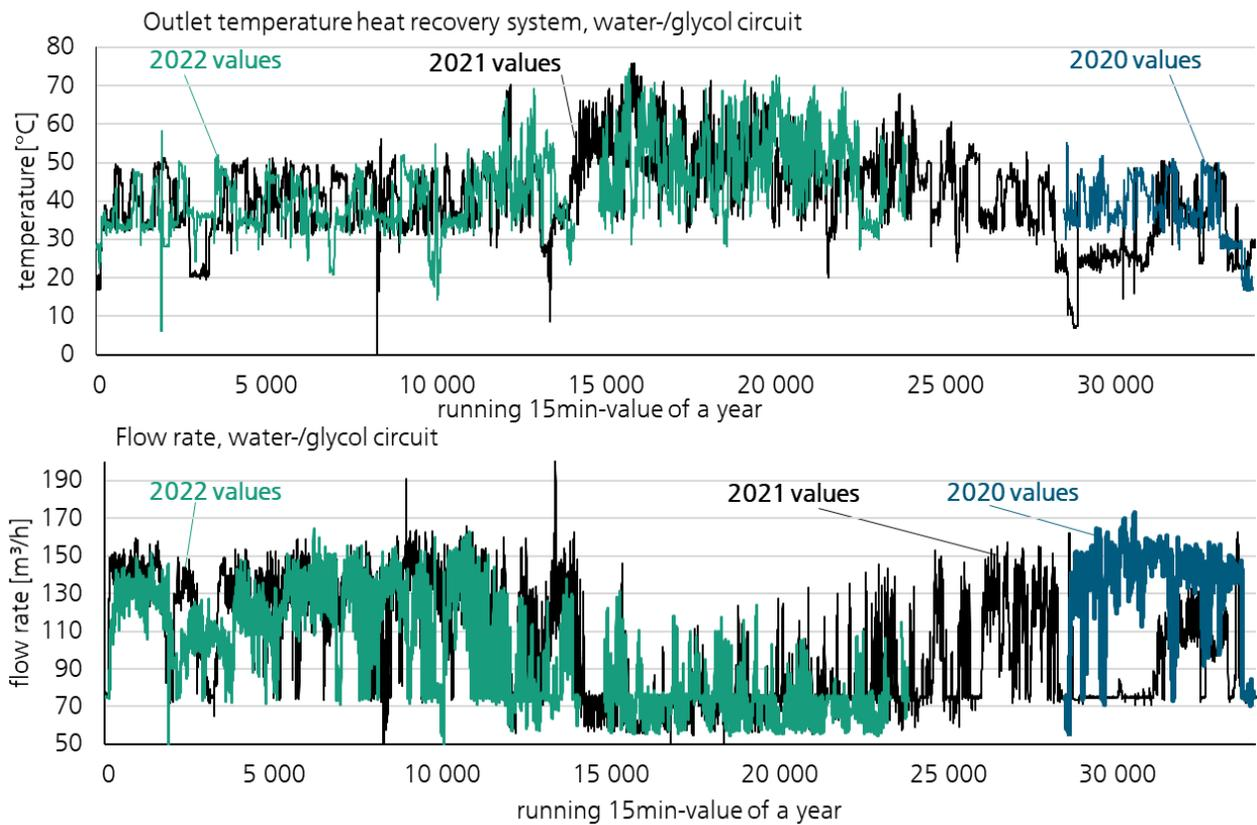
**Figure 10: Outlet temperature of the heat recovery system (top) and flow rate in the water-/glycol circuit (bottom) for the years 2020, 2021, 2022**
