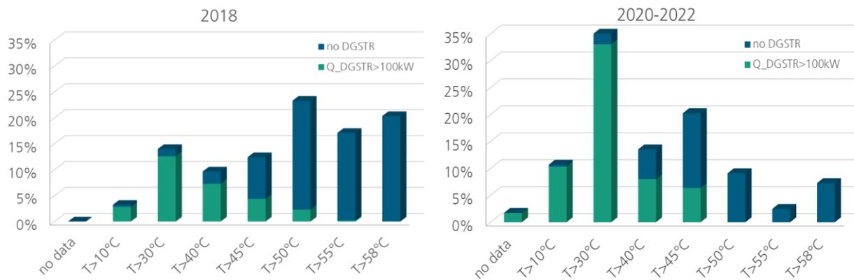
**Figure 15: Relative distribution of operating points with heat supply from DGSTR and without any additional heat demand for the time periods 2018 (left) and 2020-2022 (right) according to different water/glycol outlet temperatures of the HRS system**
