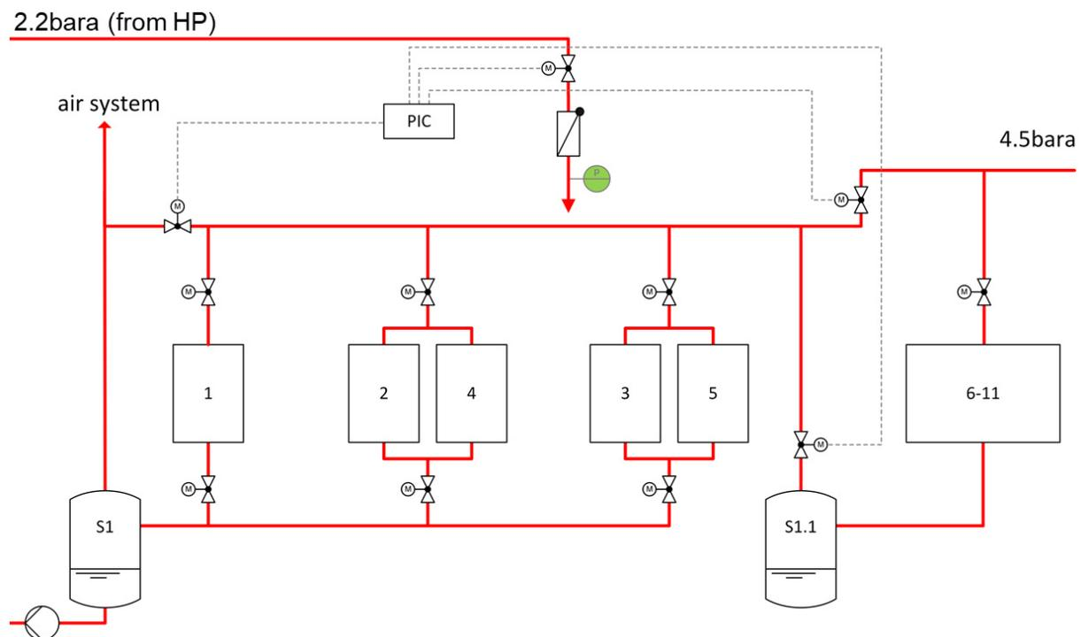
**Figure 20: First dry section (can 1 to 5) and supply line from Heat-Pump**
