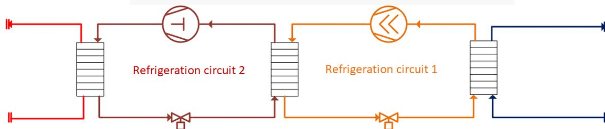
**Figure 22: Simplified setup of 2-stage heat pump system**
