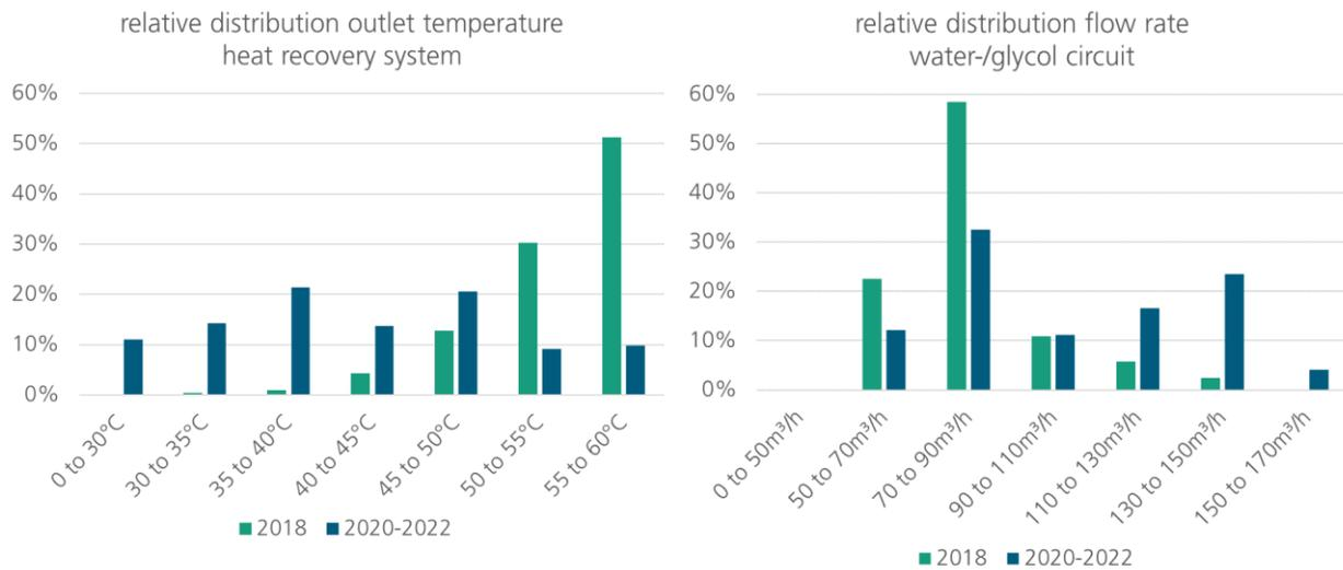
**Figure 14: Relative distribution of the outlet temperature heat recovery system (left) and relative distribution of the flow rate in the water-/glycol circuit (right) for the time periods 2018 and 2020-2022**
