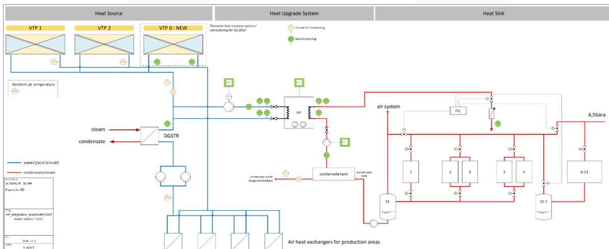
**Figure 23: Functional P&ID Scheme for the heat upgrade system in the demo site 1 in Weißenborn**
