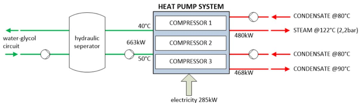
**Figure 8: Initial heat upgrade system of the STC paper factory in demo site 1**
