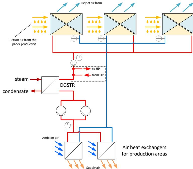
Figure 21: Selected hydraulic integration for the HUS into existing HRS (see dotted box)
