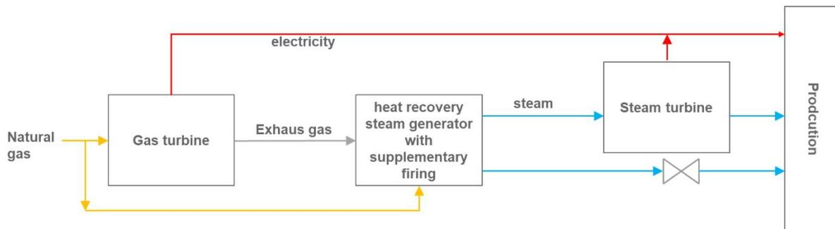
Figure 4: Combined Heat and Power (CHP) supply on site
