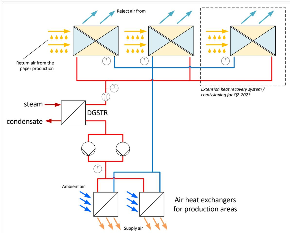
**Figure 9: Simplified setup of the water-glycol-circuit and the heat recovery system**
