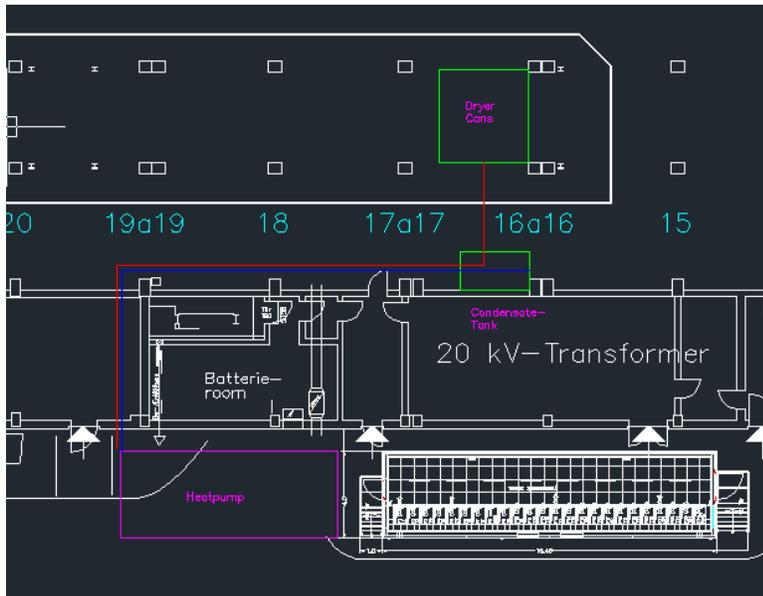
**Figure 24: Layout of heat pump installation in Weißenborn (Container = 3 m x 10,5 m) and foreseen integration points into the heat sink (blue line: condensate, red line: produced steam)**
